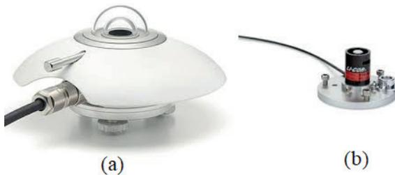
FIGURA 42: Piranômetros: (a) Eppley; (b) LICOR
